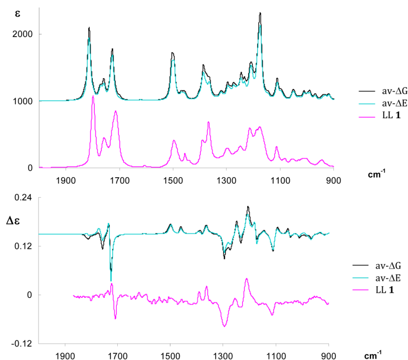
Figure 7. Comparison of experimental IR (top) and VCD (bottom) spectra of 1 with the corresponding Boltzmann average calculated spectra.
